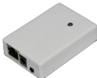
To control infrared equipment, Soline uses a universal remote control that can be controlled via the computer network. Such a remote control can control all the equipment that is in its field of vision or up to six different pieces of equipment if the module is «hidden» in a wardrobe. The user can control it with simple commands such as «Soline, I want to watch BBC» or «Soline, next channel».
